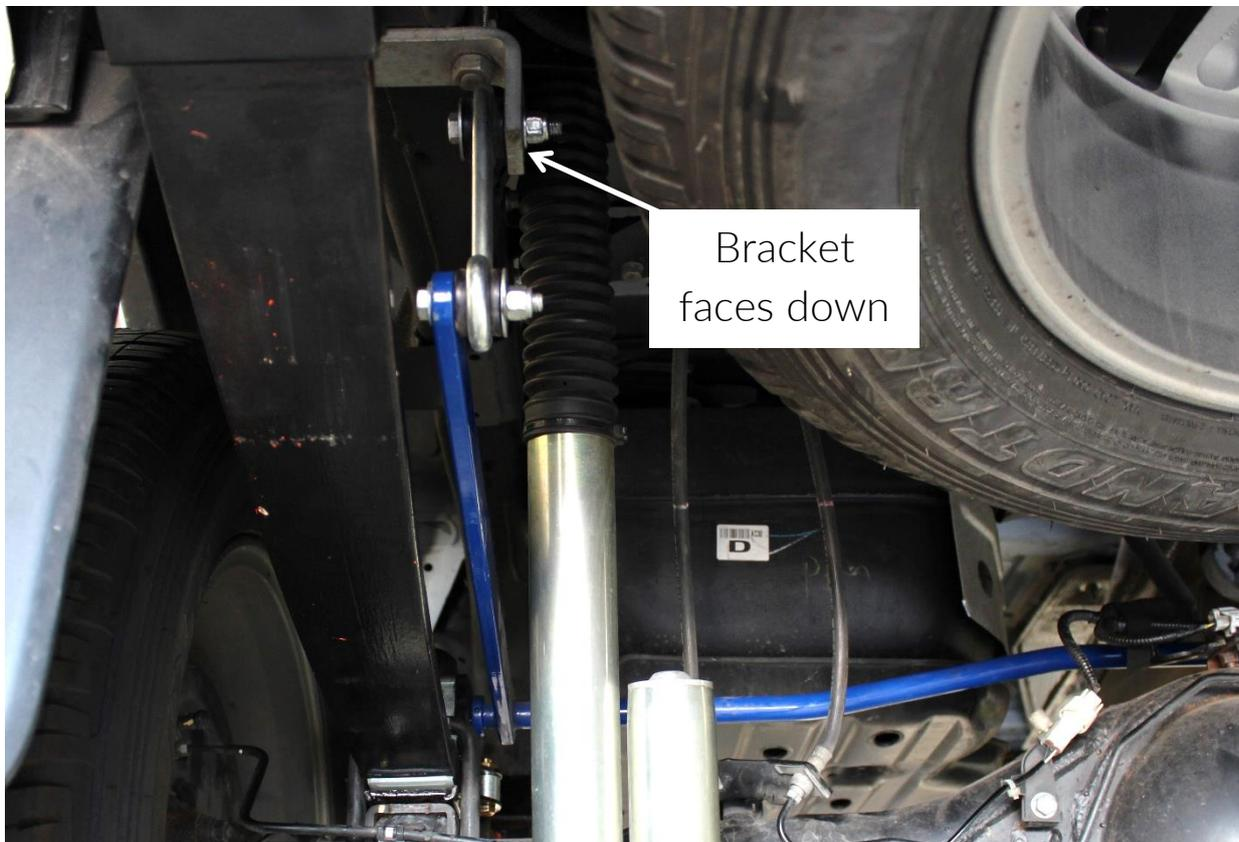
Figure 1 - Sway bar installation.
