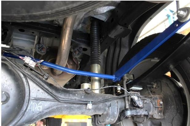
Figure 2 - Sway bar installation.
