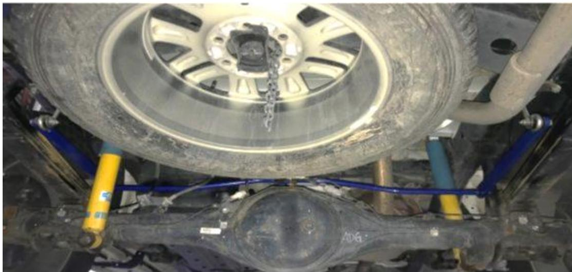
Figure 4 - Sway bar installation.
