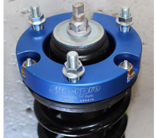
Picture 1: Picture of strut spacer on strut
