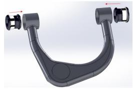
**Note**: Bushings must be pressed in with the shell side of the bushing facing. outwards from the control arm as shown.
