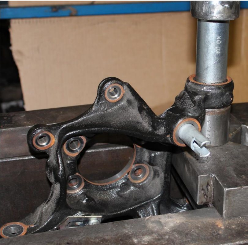
Figure 3: O.E Bush Removal from the rear hub
