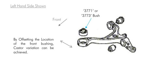
*Note:* Polyurethane bushings must be fitted to both sides of the vehicle.
