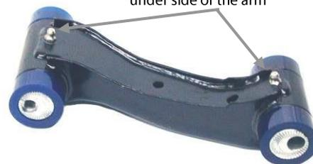
The grease nipples allow you to lubricate the bushes after installation of the arms and this also ensures the bushes are lubricated correctly after the arm is installed.
