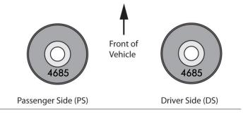
**Kit #4686K** – To counteract a slight pull to the left Single Offset, Passenger side caster increase (+0.5 degree).
