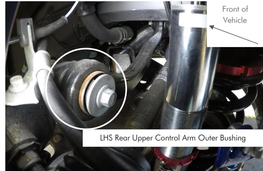
Figure 01 – Left Hand Side Upper Control Arm
