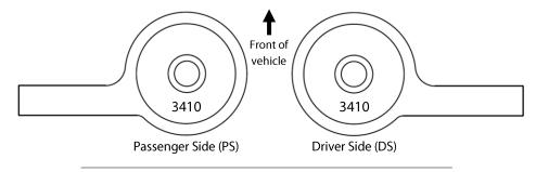
**Kit #3411K** – To counteract a slight pull to the left (approx. 0.8 deg. change) Single Offset – Passenger side castor increase & drivers side no castor change.
