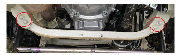
3. Install the new cross member with the longer crush tube section facing forward, as shown below.
