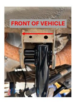
4. Re-install the OEM bolts and nuts and tighten them to OE specifications.
