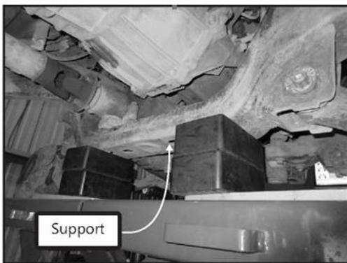
Figure 1- Recommended Chassis Support
