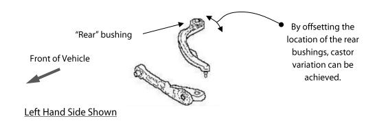
**Note:** Polyurethane bushes must be fitted to both sides of the vehicle.
