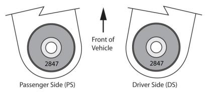
**Kit #2848K** – to counteract a slight pull to the left (Approx. 0.6 deg. change) Single Offset – Passenger side castor increase & drivers side no castor change.
