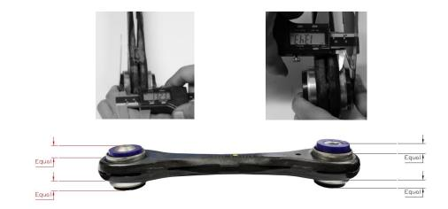
**Note:** Because the tapered end of the crush tube extrudes away from the bush (3955 only), while centralising the bushes in the arm, please ensure that you measure from the end of the crush tube to the face of the housing (As shown in figure above).
