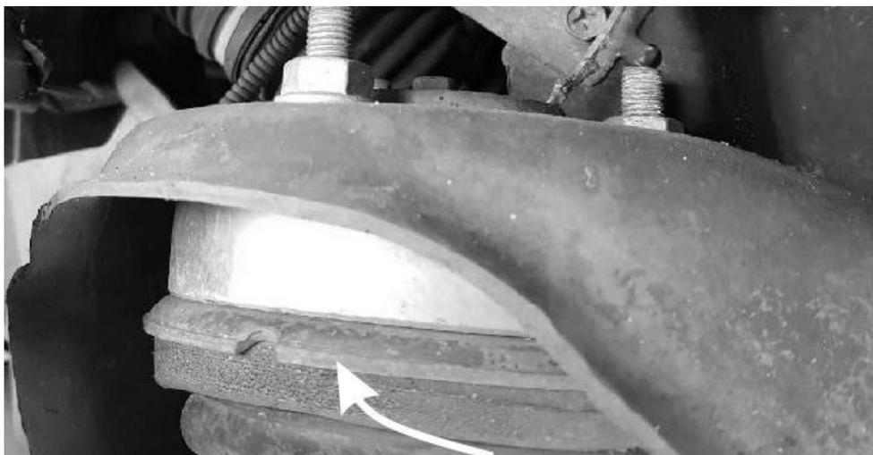
Figure 3: Example – strut-top spacer
