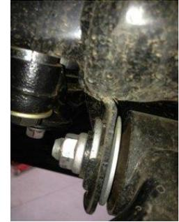
6mm spacer installed into diff mount under passenger side of vehicle (side view)
