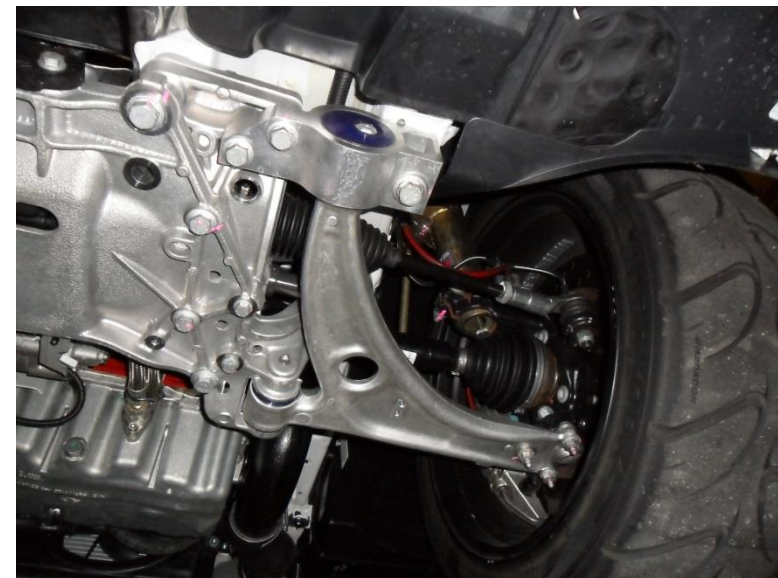
View of underside of car right hand side shown with arm assembly installed
