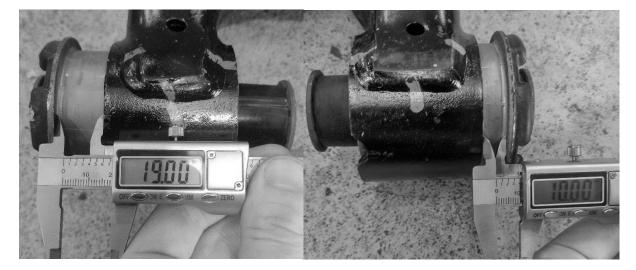
Remove OE rubber bushes from the arm either using a press and press tools or by cutting the steel shell
