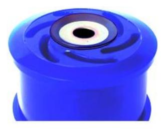
If a hydraulic press is not available, and the original bushings have been removed by other means.... the new parts can pressed into place with a large bench vice, a G-Clamp, or drawn into place with a section of threaded rod with nuts and large washers.
