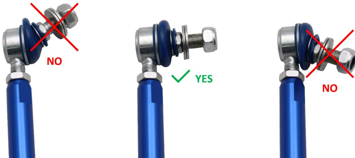
Figure 1 - Sway bar link ball end positions
