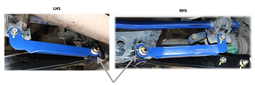
Note that the supplied <u>5mm washer</u> should be between the bracket and the sub-frame, as indicated on the picture.
