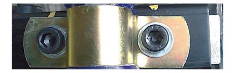
Swing the bar up towards the rear and fit the sway bar links, bolts, nuts and washers provided. We recommend the middle hole is used initially.
