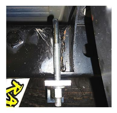
o Slide the 2 Flat plates with the 3 threaded holes into the bracket mounts on the diff.
