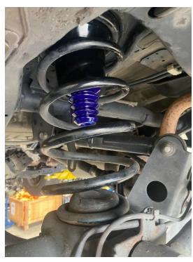
Figure 01 – Completed Installation of Bump Stop
