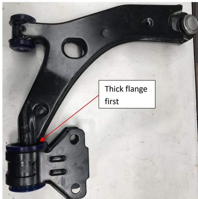
For the right arm the bracket should be in the opposite orientation as shown with the thinner part of the bush being pushed onto the arm first.
