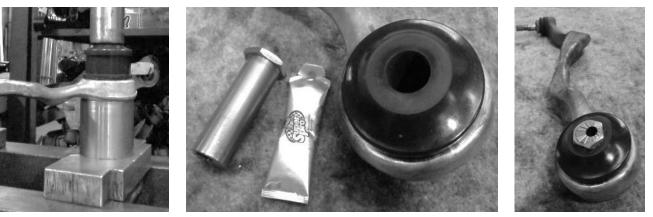
Figure 1: SuperPro Polyurethane Bushes and Crush Tube Assembly in Arm
