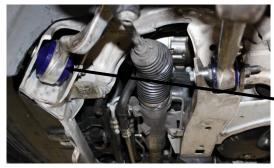
Figure 2: Radius arm assembly in chassis
