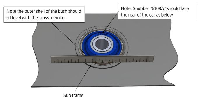
View of installed bush looking from the rear of the vehicle
