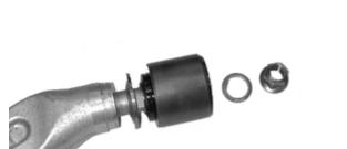
**Photo 1** – Shown in picture: Left hand side control arm, original nut and "D" washer, offset SPF2026 bush (with crush-tube inserted), supplied washer (flat).
