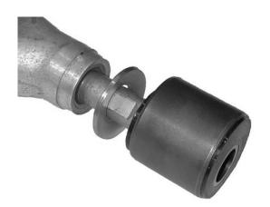
**Sketch** – To increase caster\*, press in the bushes ensuring that the offset is oriented towards the outside of the vehicle.
