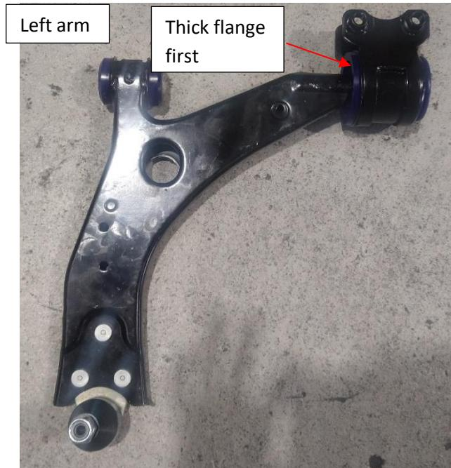
For the right arm the bracket should be in the opposite orientation as shown with the thinner part of the bush being pushed onto the arm first.
