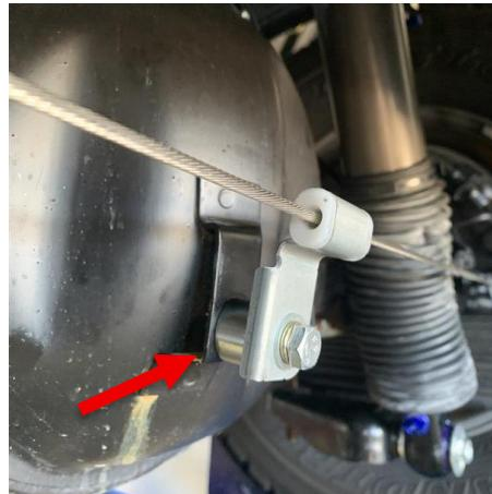
3. Remove the bracket attached to the left side of the diff housing by removing the large bolt. Once removed, free the handbrake cable by removing the center bolt.
