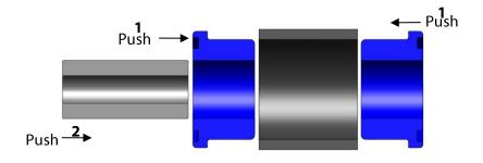
To fit the crush tube into the bushes, apply the grease supplied to the bore of the bush and the outside of the crush tube. Then, push it in;
