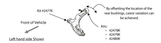
Note: Polyurethane bushings must be fitted to both sides of the vehicle.
