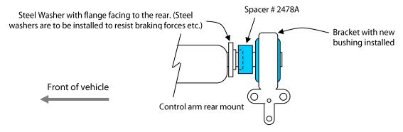
Assemble rear bushing to the vehicle as per drawing above
