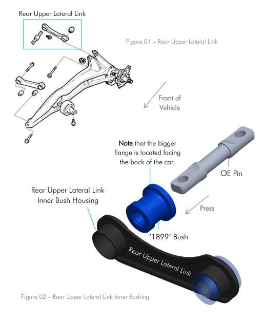
Note: Polyurethane bushings must be fitted to both sides of the vehicle. This kit should be installed by a Qualified Motor Mechanic.
