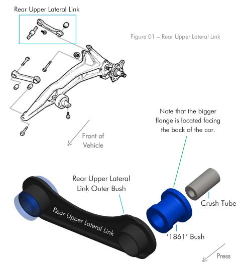
Figure 02 – Rear Upper Lateral Link Outer Bushing
