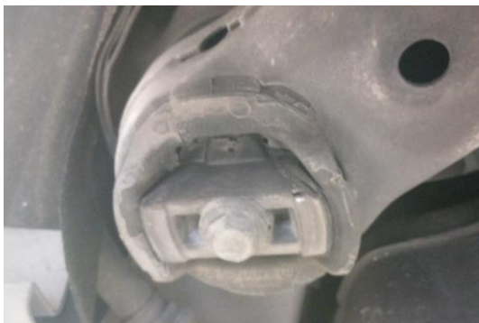
Figure 02 – Cradle Bolts to be loosened.
