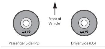
**Kit #4177K** – To counteract a slight pull to the left Single Offset, Passenger side caster increase (+0.5 degree).
