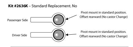
**Kit #2636K** – To counteract a slight pull to the left Passenger side castor standard & driver's side reduced to achieve castor split.
