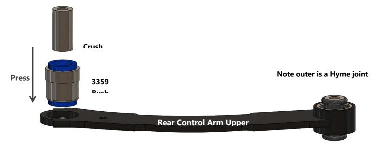
Note: Polyurethane bushings must be fitted to both sides of the vehicle. Re tension all bolts at 1000 km
