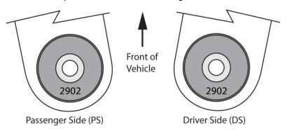
**Kit #3417K** – to counteract a slight pull to the left (Approx. 0.5 degree change) Single Offset – (passenger side castor increase & drivers side no castor change)
