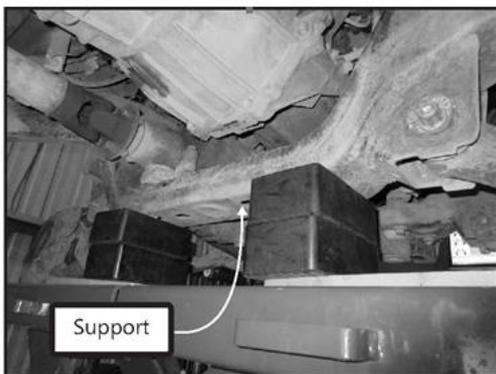
Figure 1- Recommended Chassis Support
