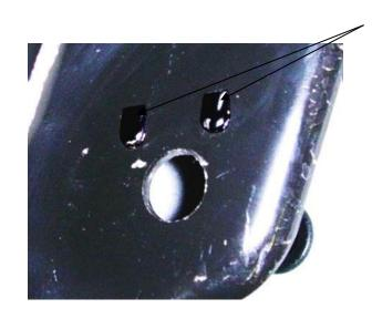
Two lugs are present above the bolt holes on each inside face of the front mounts.
