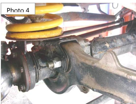
**Photo 4** – Refit the arm in the reverse order of removal, during installation check that the trailing arms have sufficient clearance between the top of the arm, and the differential housing bracket. It may be necessary to remove some of the flashing from the casting edges on the arms to provide adequate clearance.
