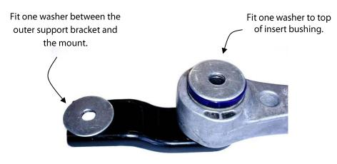
Offer the bracket to the vehicle as shown above.
