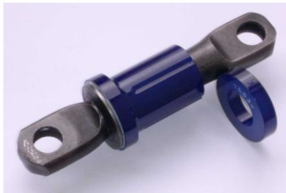
Figure 1: 4099 polyurethane bush assembly with factory tube (left), and then press into arm (right). After that, slide 2663R polyurethane bush through the pin and then, assemble the stopper on the pin.
