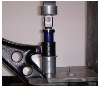
Figure 1: 4099 polyurethane bush assembly with factory tube (left), and then press into arm (right). After that, slide 2663R polyurethane bush through the pin and then, assemble the stopper on the pin.
