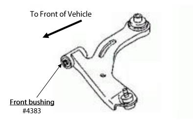
*Note:* Polyurethane bushes must be fitted to both sides of the vehicle.
