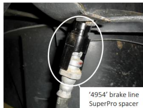
Figure 02 – Installing '4954' brake line spacer
