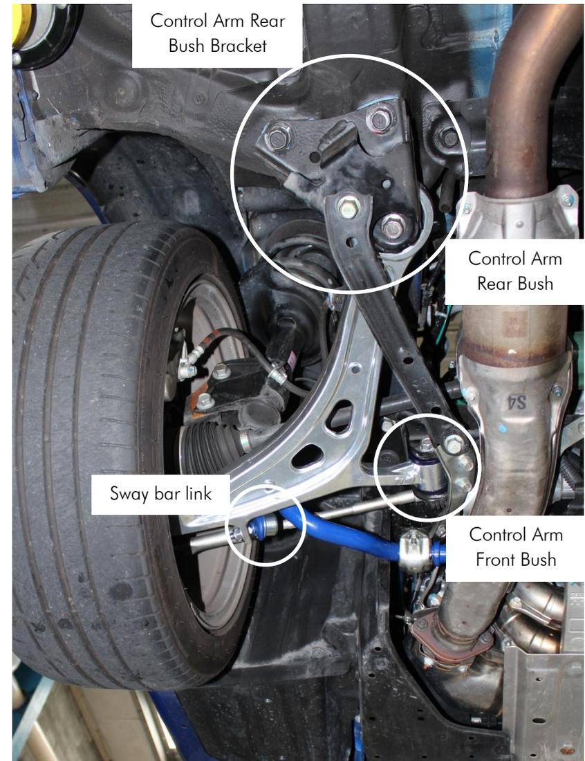
Figure 02 – View from underneath of the vehicle - Right Hand Side Control Arm assembly installed
