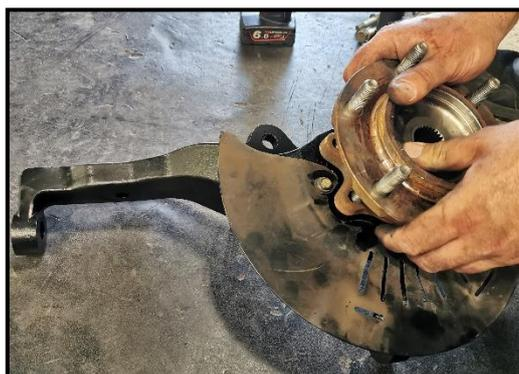
Figure 6: Remove wheel bearing hub assembly & dust shield
