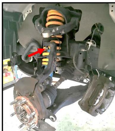
Figure 4: Loosen nut but do not remove, this will keep the steering knuckle from falling.
