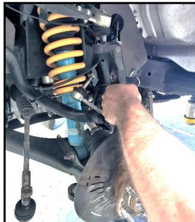
Figure 5: Remove OE steering knuckle from the vehicle
