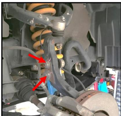
Figure 1: Remove brake line bracket & Swaybar Link
