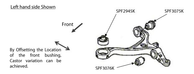
**Note:** Polyurethane bushings must be fitted to both sides of the vehicle.
