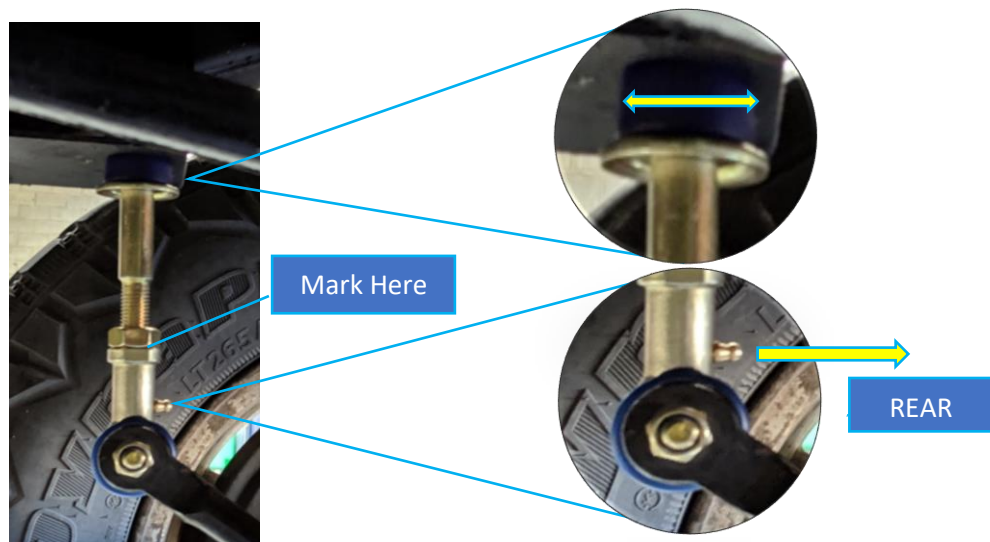
Figure 2. Installed Rear Driver's Side Link Pin
