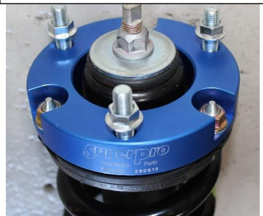
Picture 1: Picture of strut spacer on strut
