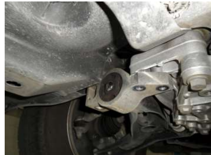
Fig 1 Remove Front lower control arm bolts and Rear bracket bolts
