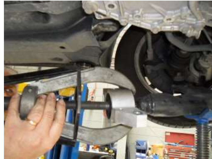
Fig 3 – Extract bush / bracket off arm using bearing puller or similar
