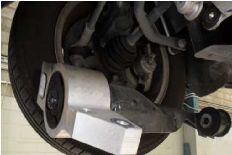
Fig 2 – Arm in lowered position note ball joint still attached (Left Hand Shown)
